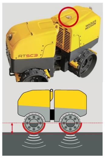
Below the axle exciter in each drum: means more efficient transfer of compaction energy to the soil and improved stability of the machine.
