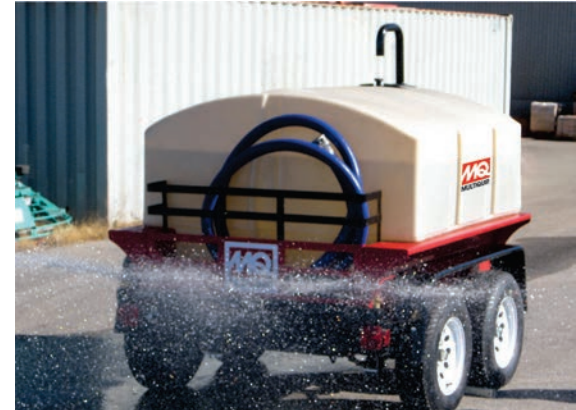
Rear spray bar produces a 30' cone pattern using water pump pressure or a 9' cone under gravity pressure.
